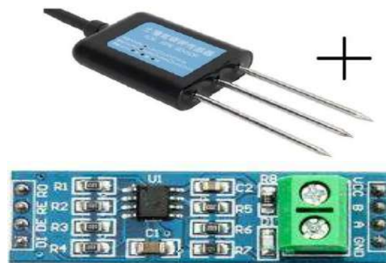
MAX485 RS485 Transceiver Module
